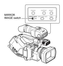
When the camcorder is in Media mode, the picture is also inverted both vertically and horizontally. In Camera mode, the picture is inverted only vertically, while it is also inverted horizontally for Rec Review (page 74).
